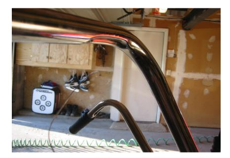
Pull all of the hand grip wiring out of the bike, not back to the bars.
