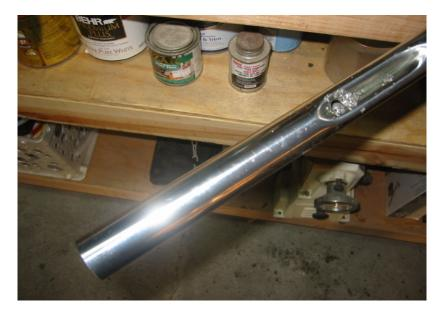
Put the handle bars in your vice. I used wooden blocks to keep from scratching the bars while drilling.
