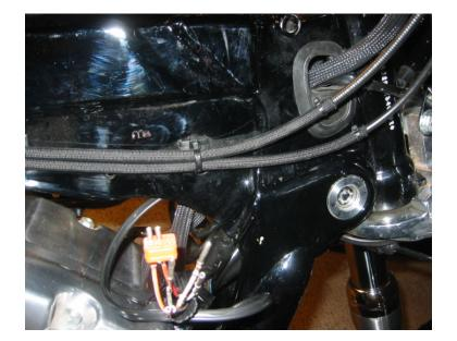
Route the wires back through the bike. I electrical taped mine to keep them together so that I could "thread" them back through. Its tight with all those wires.
