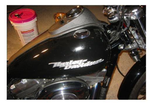
Finish removing the gas tank. Disconnect the tube that allows the gas to flow from the left side to the right side. Make sure your container is large enough to catch all the gas. Cleanup all spilled gasoline.
