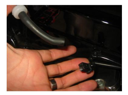
Remove the bolts that hold the tank on, disconnect the fuel gauge and the gas escape line from the fuel tank. There should be nothing holding the tank on now, just remove it. If you didnt drain all the gas you will spill some more all over.
