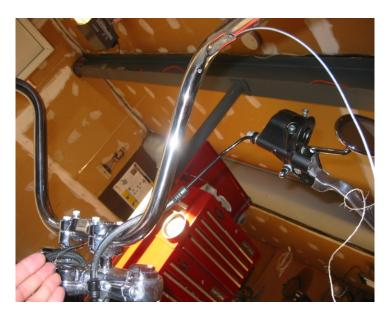
I ran a small flexible wire through the holes. I then attached the small flexible wire to the hand grip wiring and slowly (slowly) fed it through while pulling and pushing the wires. I was able to feed the wires and the plastic sleeve through the handlebars all in one shot. It was really tight but I just took my time and tried to be very careful not to bind against those sharp edges I filed down.
