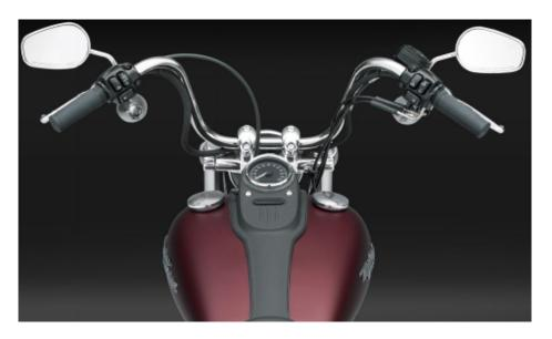
A riders view of the wires. On the left hand grip they are the ones closest to the ground. The right grip has the wires, the throttle cables and the front brake line
