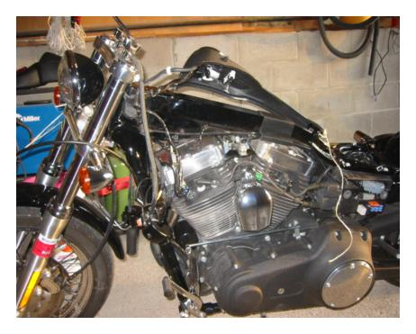
Shim the brake lever according to the service manual. I used a small piece of cardboard. Remove the hand controls. Be careful not to strip the torx bolts. They are two different sizes (t25 and t27) however I didnt have a t27 torx bit, so I was just real careful. Remove the handlebars. Pull all the wiring out from under the frame so you can get to the connectors.
