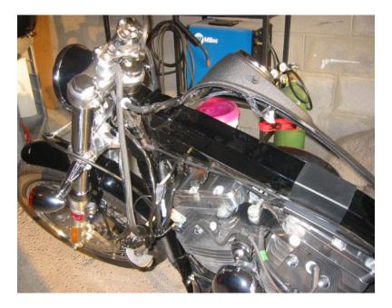
One last shot of the stripped bike. One thing I did do differently than the last time I took the bike apart: I tied a small piece of twine to the brake master cylinder and to the ceiling of the garage. This kept it upright and kept any brake fluid from leaking out.
