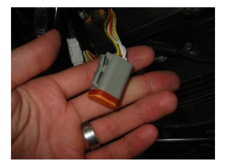
Locate the deutsche connectors for the handgrip wiring. Carefully note where each wire goes. mark the connector itself on your diagram and on the connector itself so you will be sure to orient it properly in reassembly. Refer to your service manual to take them apart. If you dont have one, pry the orange cover off with a flat head (carefully) then use an exacto knife to pry up the prongs holding the wires in place. One by one, remove each wire.
